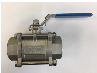
2" BSP full flow stainless steel 3 piece ball valve with PTFE seals
