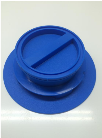
3" Discharge Gland Assembly (with cutter and membrane) Comprises of MET0000085 3" Gland (Blue) 3" BSP Internal Thread (Female) MET0000084 3" Crown Cutter (Blue). MET0000088 3" Blue Nitrile 'O' Ring 82.22mm x 2.62mm MET0000086 3" BSP Male Plug (Blue) MET0000267 Membrane Rolls LLDPE Laminate 112mu (BLUE)
